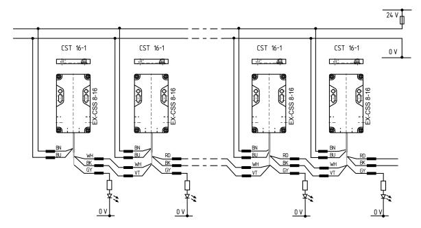
BK and RD = safety outputs Y1 and Y2  $\rightarrow$  safety-monitoring module
